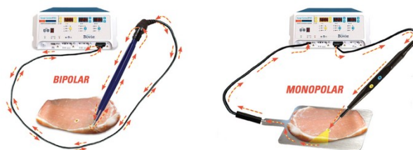
Figure 4: Figure showing the difference between monopolar and bipolar electrosurgery
