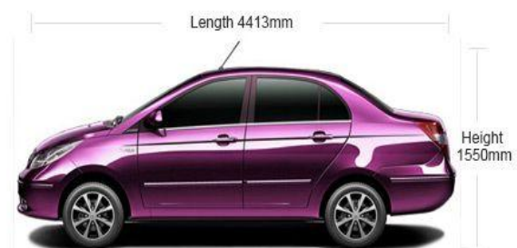
Figure 4: Dimensions of the generic vehicle model [Side-view]
